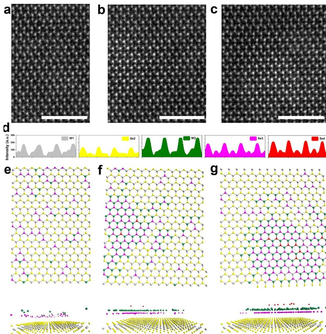
**Figure 3.** a-c) Atomic resolution Z-contrast images of monolayer WSe<sub>2</sub>. d) Intensity profiles of different atom clusters. e-g) The atomic structure determined by the histogram analysis corresponding to images a (e), b (f), and c (g), respectively.
