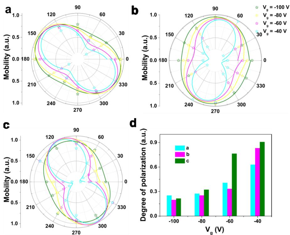
**Figure 5.** a-c) Polar plots of angle-resolved carrier mobility for three WSe<sub>2</sub> FET devices with the gate voltage at -100 V, -80 V, -60 V, and -40 V. d) Histogram of anisotropic degree of carrier mobility from the three WSe<sub>2</sub> FET under different gate voltages.
